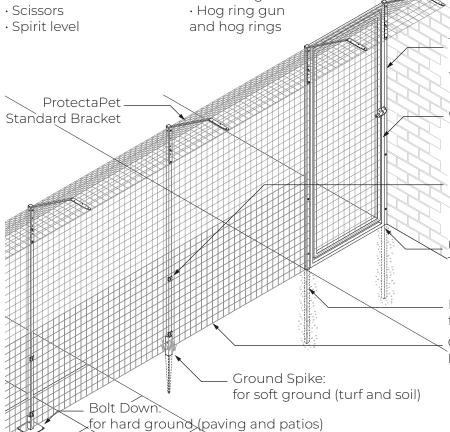
The standard wall end fixing method (without a gate) is the hook & wire frame. See step 12 & 13 for installation method
