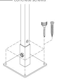
Bolt posts to either side of the gate assembly using coach bolts & nuts supplied
