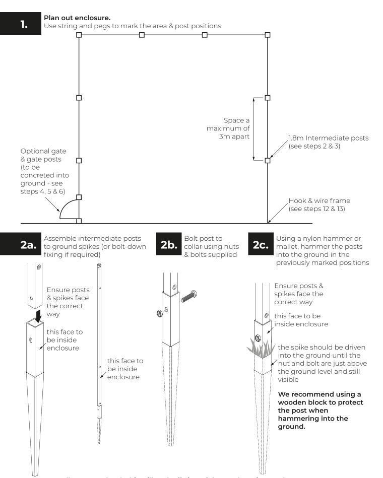
TIP: Ensure all posts are level. This will make fitting of the mesh easier at a later stage.
